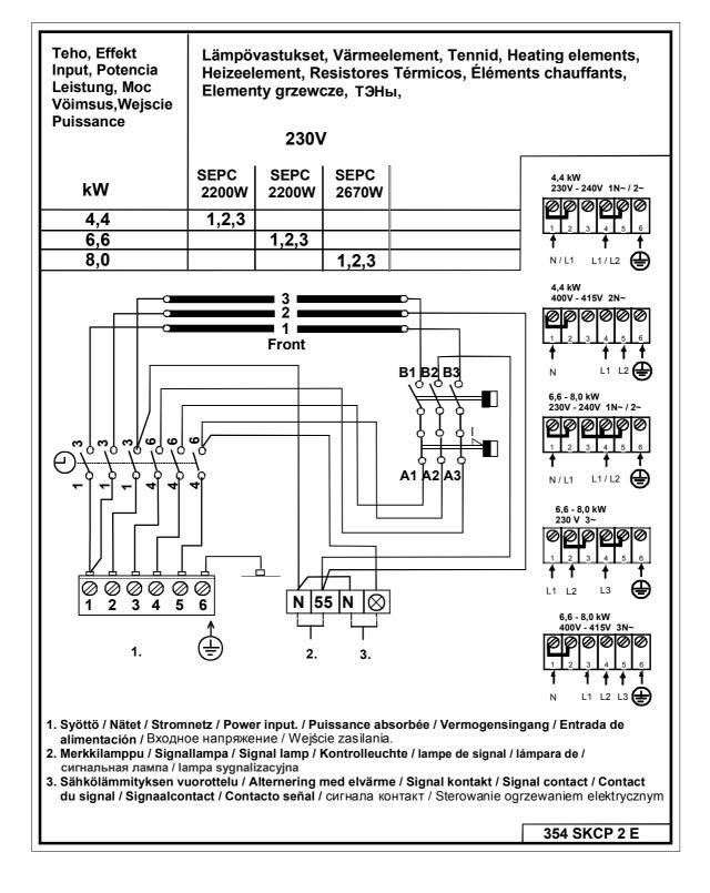
Image 4 Switch diagram for the sauna heater
